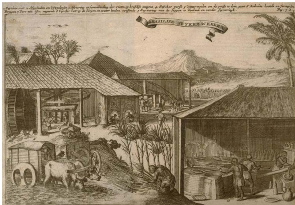
Figure 1. Condensed portrayal of a Brazilian ingenio complex, showing all of the stages of a sugar-making operation. Notes: Grinding mills are left and center, and are powered by water and animal power. Meanwhile the boiling, striking, and curing aspects are portrayed on the right. Question: What is the diagonal box for in the picture? Another pair of mills are portrayed in the distant background. Source: Image initially from Simon De Vries, Curieuse aenmerckingen der bysonderste Oost en West-Indische verwonderens-waerdige dingen . . . (Utrecht, 1682); used with permission from the James Ford Bell Library, at the University of Minnesota.
